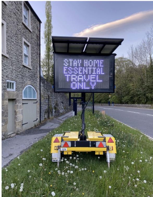
VMS-A – portable trailer based mobile Variable Message Sign
